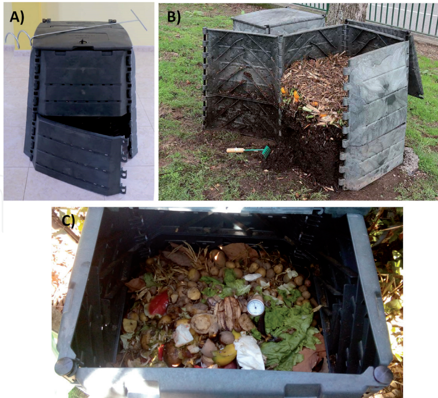
Figure 2. (A) Home composter with an aerator on the lid, (B) material in composting process (C) bio-waste feeding to the composter and temperature measurement.
