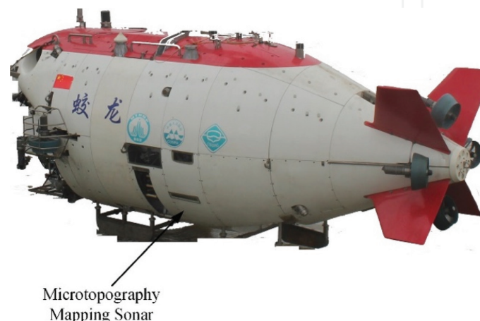
Figure 7. Human-occupied vehicle Jiaolong.
