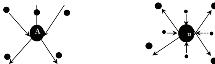
Figure 2. Hub and spoke for a flight network pattern. A: Hour glass hub & spoke. B: Hinterland hub & spoke.
