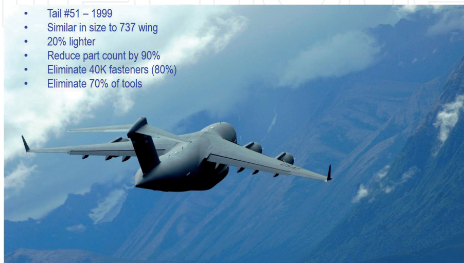
Figure 15. C-17 horizontal stabilizer.
