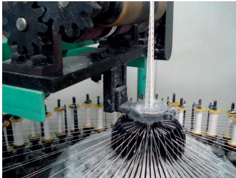
Figure 12. Accumulation of broken fibers at fell point due to beatup knife abrasion.
