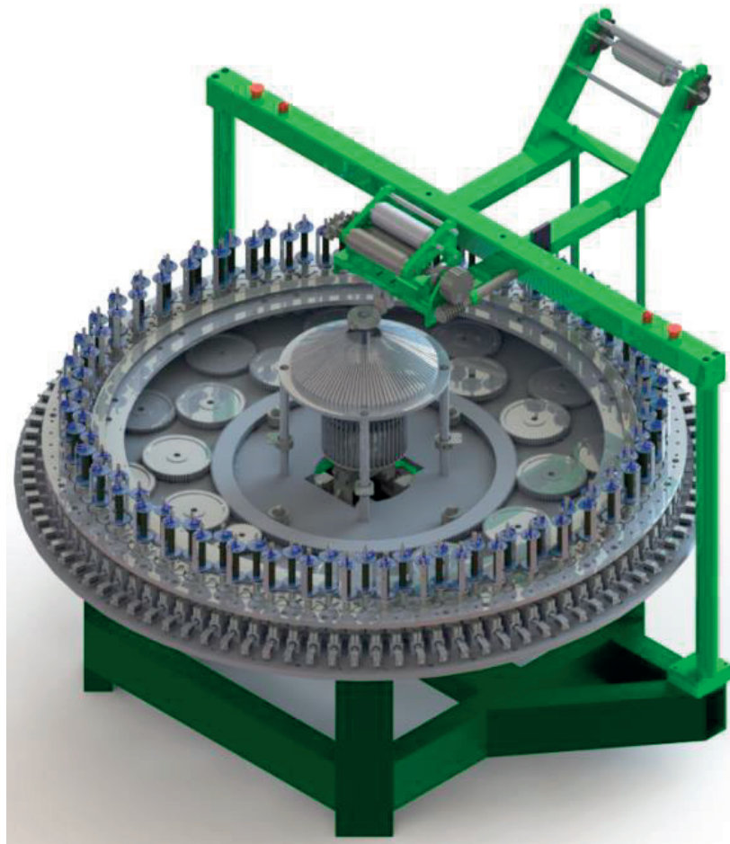
Figure 5. CAD drawing of modern lace braiding machine.
