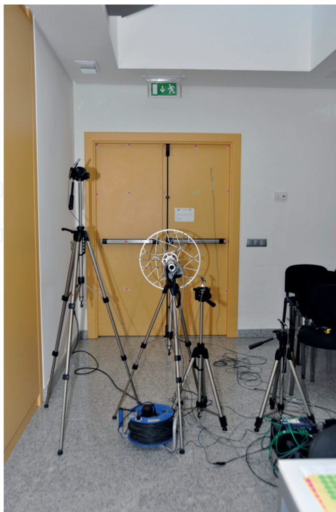
Figure 3. Example of the beamforming measurement layout.
