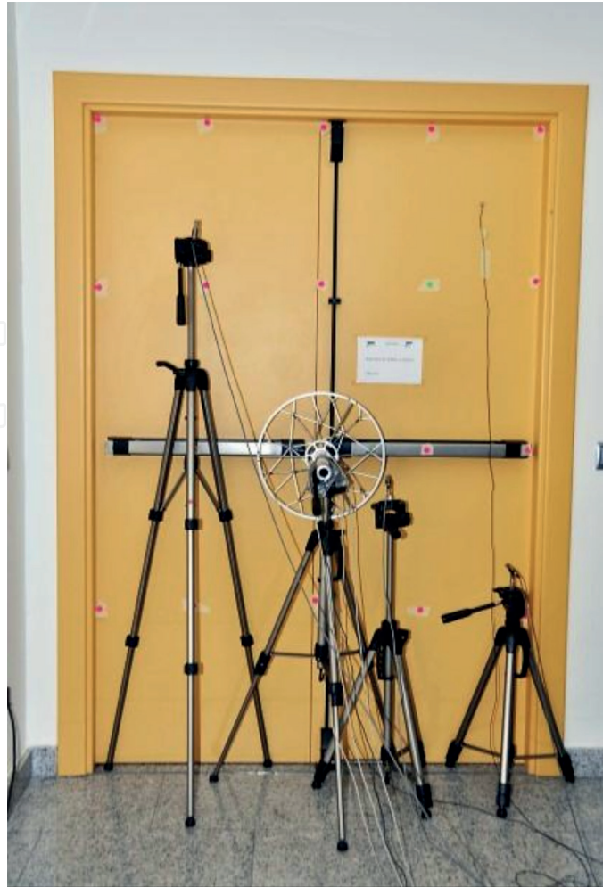
Figure 4. Example of the SONAH measurement layout.
