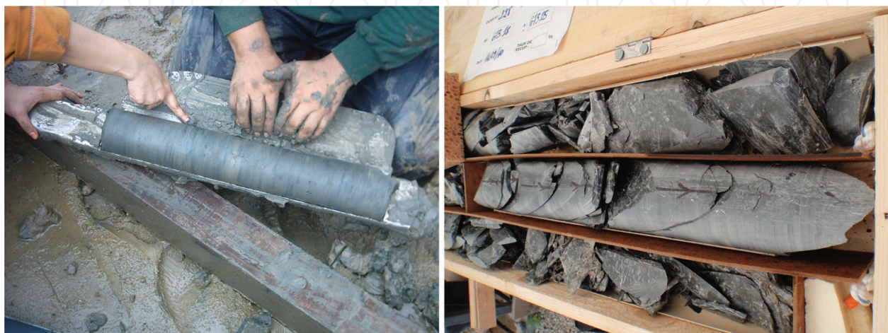
Figure 7. Core sample collected from mangrove environment used for metals proxy study. Photo by Ong Meng Chuan.
