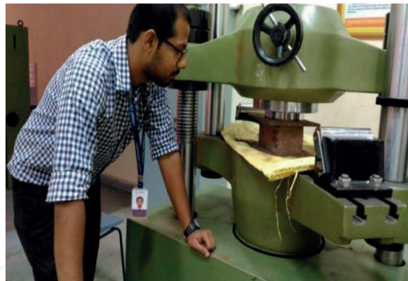
Figure 1. Compression test of geopolymer bricks.
