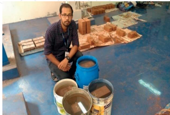
Figure 2. Water absorption test of geopolymer bricks.
