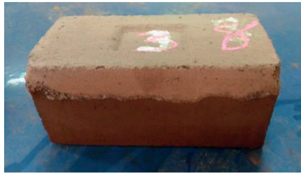
Figure 5. Efflorescence test of geopolymer bricks.
