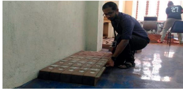
Figure 3. Dimensionality test of geopolymer bricks.
