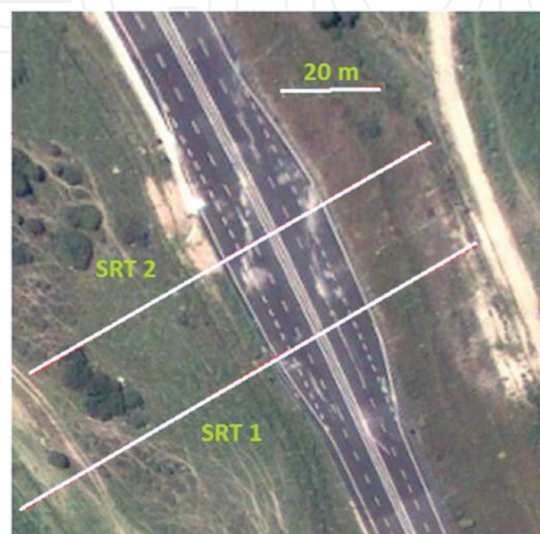
Figure 13. Position of the two seismic refraction tomographies.
