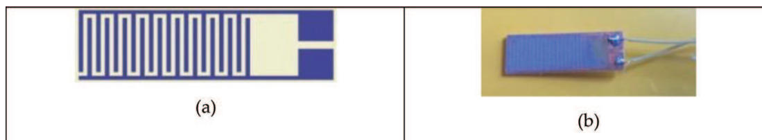
Figure 21. The NO 2 gas sensing element structure (a) PCB substrate with interdigitated Ag array electrode; (b) the sensing element made with PCB substrate and sensitive material deposited on surface electrode.
