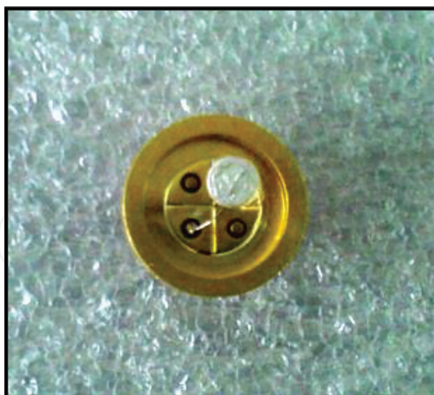
Figure 1. Image of the CO 2 sensor made with mixed oxides CeO 2 -Nb 2 O 5 sensitive material.
