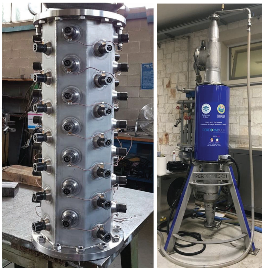
Figure 2. The inner part of the sono-heat-exchanger (on the left). The external structure of the sono-heat-exchanger (on the right).
