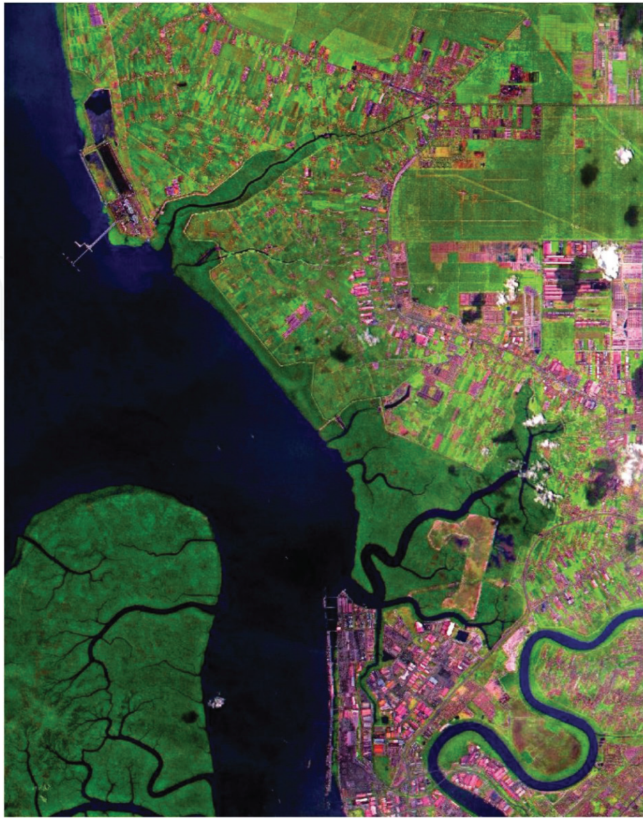
Figure 6. Mangroves as they appeared on Landsat-8 image. The dark green areas represent the mangrove areas. The image classification process, either automated or manual digitizing, is usually easier for mangrove areas than for other vegetation. The image is displayed using a combination of bands 543 (RGB) over the Kapar area in Klang, Selangor. The central bottom is Klang port complex and the bottom left is Pulau Klang, which is predominantly covered by mangroves.
