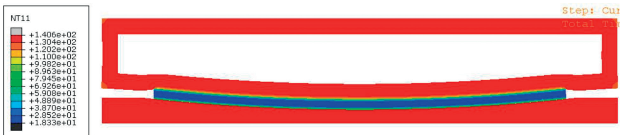
Figure 13. Nodal temperature results at t = 120 s (relative to current load step).
