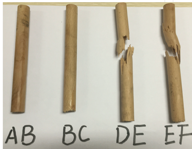
Figure 19. Failure of connectors in SPT-G3-16.
