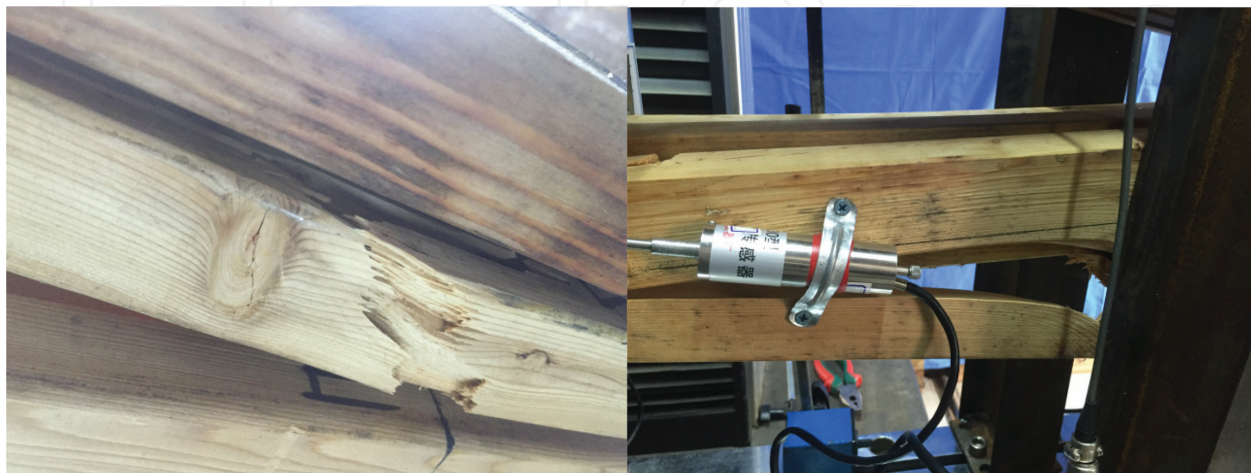
Figure 18. The failure of SPT-G3-16.
