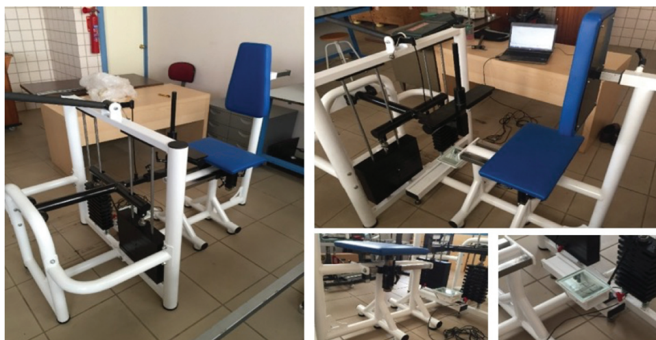
Figure 4. Pictures of the measuring device that integrates the different elements (regulation systems, load cell, and integrated software) to obtain the mechanical properties of the plantar flexors by means of the free vibration technique.
