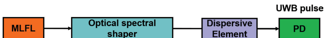
Figure 7. The block diagram of a UWB-IR generation system based on optical spectral shaping and frequency-to-time mapping. MLFL, mode-locked fiber laser.
