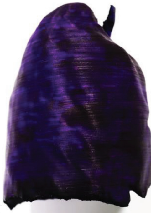
Figure 13. Final 3D printed model of a lung painted with acrylic paint.
