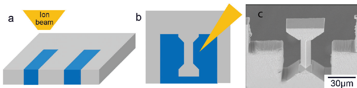
Figure 12. Schematics of tensile specimen fabrication. (a) Rough milling, (b) fabrication of grip part, and (c) SEM image of tensile specimen after gauge part milling by non-tapered pillar fabrication procedures.
