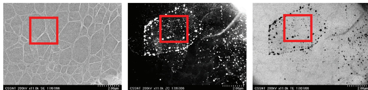
Figure 5. Co-localized SE—secondary electrons (left), ZC—phase contrast (middle) and TE—transmission electrons (right) images of the Au/rGO y sample.
