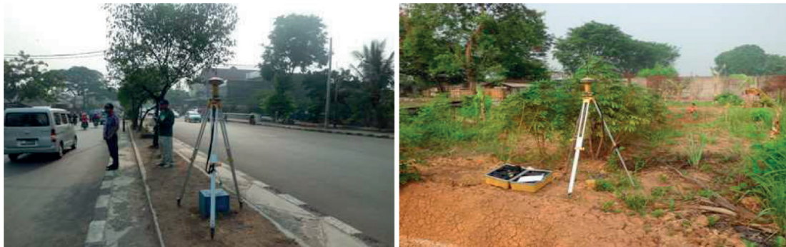
Figure 2. Field survey GPS observation to derive land subsidence (source: authors).
