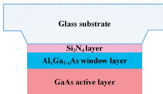
Figure 3. Structural schematic of multilayered t-mode GaAs cathode module, including the glass substrate, the Si 3 N 4 antireflection layer, the Al x Ga 1-x As window layer, and the GaAs active layer.
