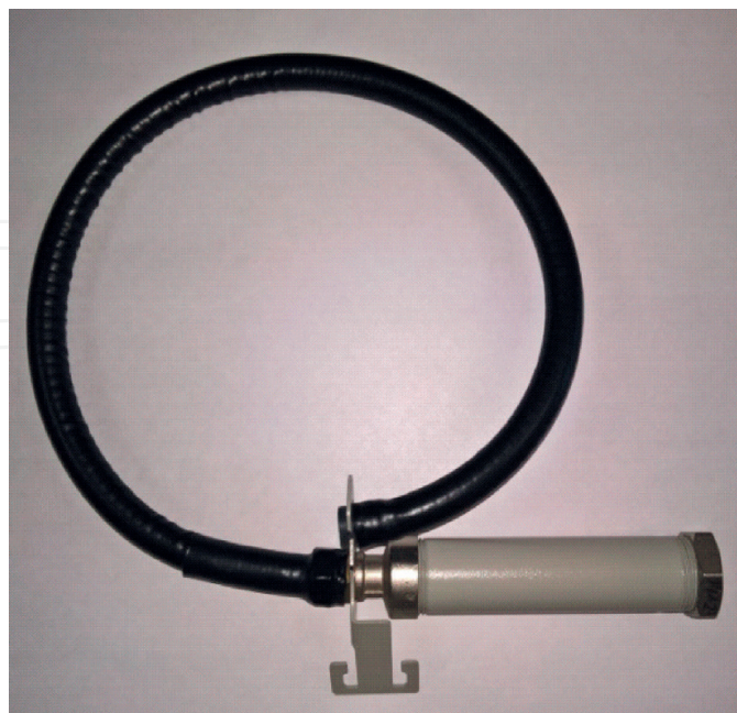
Figure 15. Photo of the device for registration of current derivative from the source of powerful EMI action in the near field based on the 4th generation lightning current recorder.
