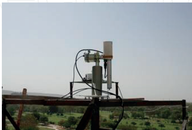
Figure 3. The CIMEL Sunphotometer instrument.
