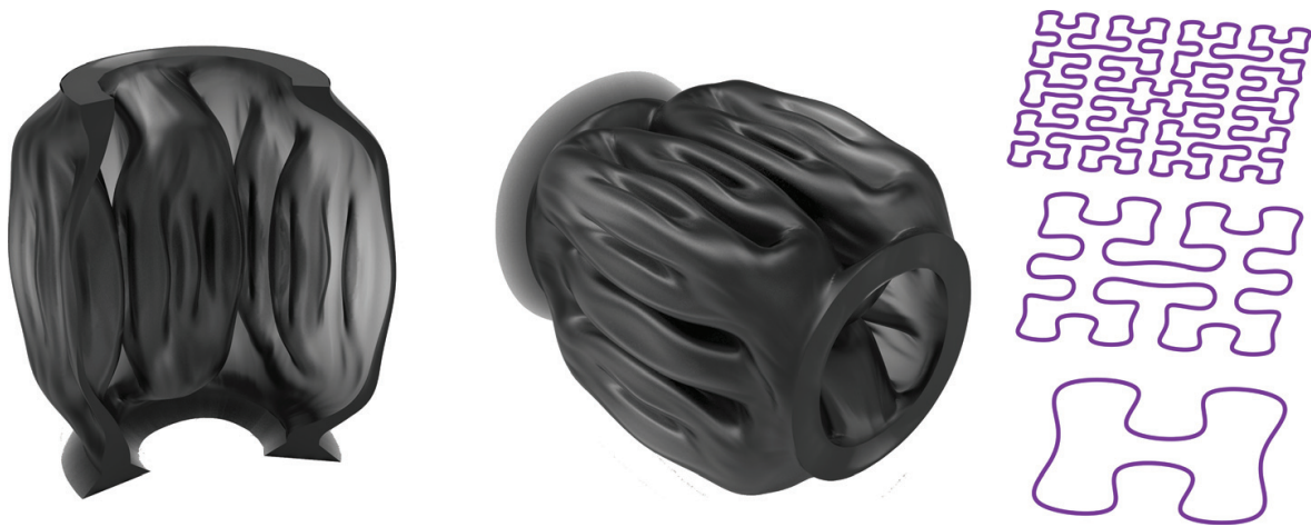
Figure 14. Alternative structure as a concept for a heat exchanger. From left to right: a 5/8 cutout to show the inner structure; the whole component (lying); the curves used for designing the structure.
