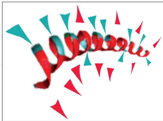
Figure 3. The distribution of hydrophobic residues along the helix does not correspond to its structural periodicity. The image schematically depicts the expected reaction of the surrounding water particles, which are either attracted (teal) or repelled (red) by the molecular surface.
