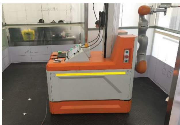
Figure 24. MoMaCo (mobile manipulator in construction).
