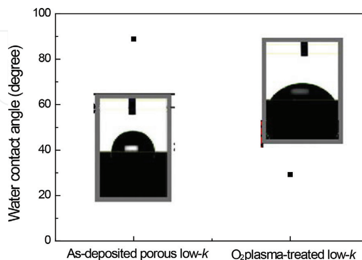
Figure 4. WCA values and images of porous low- k dielectrics after O 2 plasma treatment.
