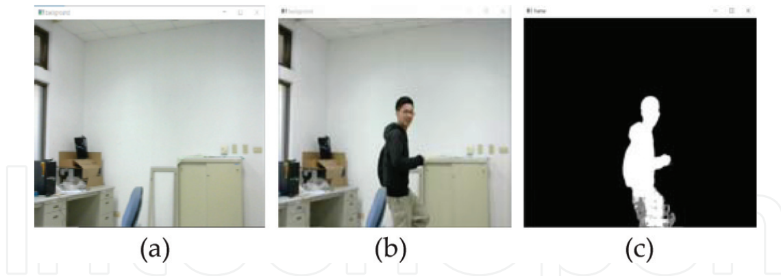
Figure 3. Foreground pixels representing the moving objects obtained by the adaptive Gaussian mixture model: (a) background, (b) moving object, and (c) foreground pixels.
