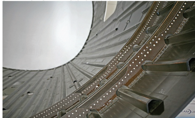
Figure 2. Disassembled composite fuselage section of the Boeing 787.
