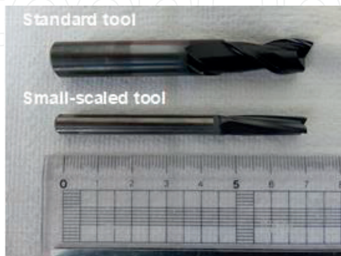
Figure 8. Two diamond-coated end-milling tools as a specimen for plasma ashing process.
