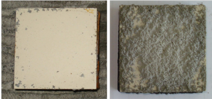
Figure 7. 9. Examples of cementitious-adhesives failure patterns commonly observed in the actual study (left image – AF-T observed on samples cured in water; right image – CF-A observed on samples cured under heat).
