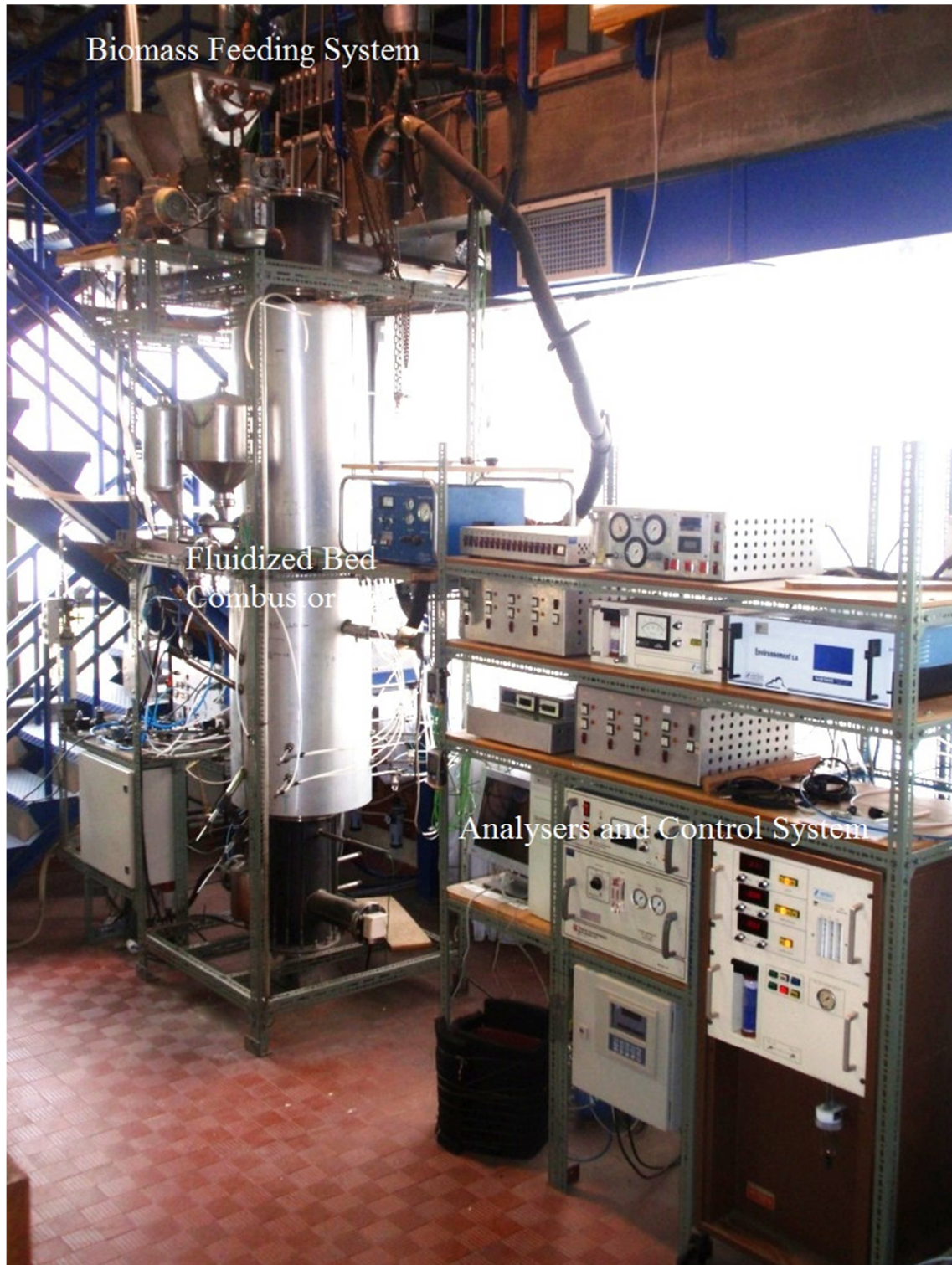
Figure 2. 2. Pilot scale bubbling fluidized bed combustor (Department of Environment and Planning of University of Aveiro, Portugal).
