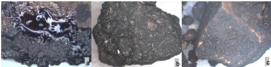
Figure 4. 4. Bituminous mixes optical microscope images: (a) MBBr (50x), (b) MBG5% (10x) and (c) MBD5% (10x).
