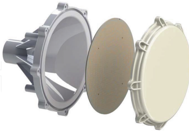
Figure 8. Perspective view of the complete transmitarray antenna [14].
