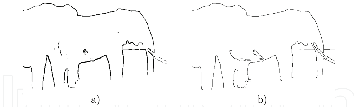
Figure 11. Edge detection: (a) memristive grid at t = 20.45 ms, (b) Canny's method [2] for a threshold 0.422.
