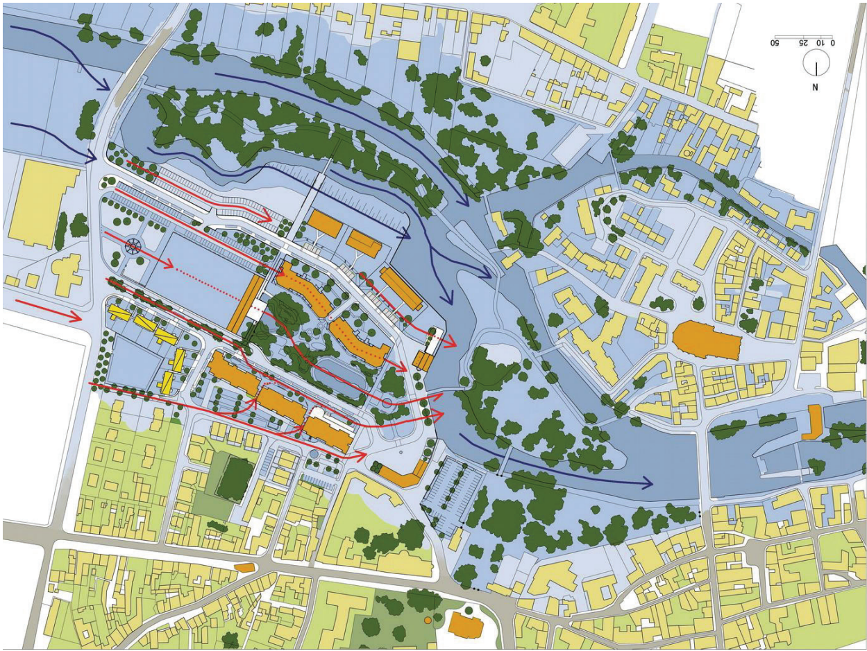
Figure 5. Romorantin, a study of hydraulic transparency during a 100-year flood in “Matra” district (the flow of water through the district marked in red). Source EDL - Eric Daniel Lacombe.
