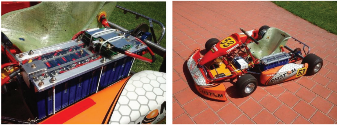
Figure 9. 48 V Lithium-ion battery pack with BMS and the prototype electric kart.
