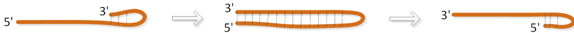
Figure 4.2 Illustration of the MFE estimation algorithm. All possible folds of a single stem-loop are considered, starting from the 3' end. In each fold, the nucleotides close to the folding region are not considered to interact. The average of the nucleotide-pair contributions of all folds is the result.
