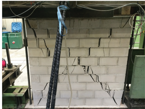
Figure 13. CS_S1: calcium-silicate brick masonry wall strengthened on one side. Cracking pattern and equivalent multilinear curve.
