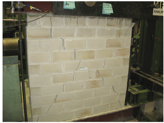
Figure 12. CS_UN: calcium-silicate brick masonry wall unstrengthened. Cracking pattern at 0.51% drift and equivalent bilinear curve.
