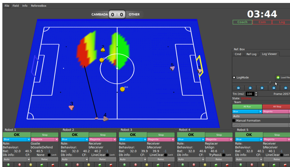
Figure 5.2: Example of alternative position map for receiver calculated for robot 2. CAMBADA is attacking to the blue goal. The black line goes from the ball to the alternative position indicated by robot 2 to receive the ball.
