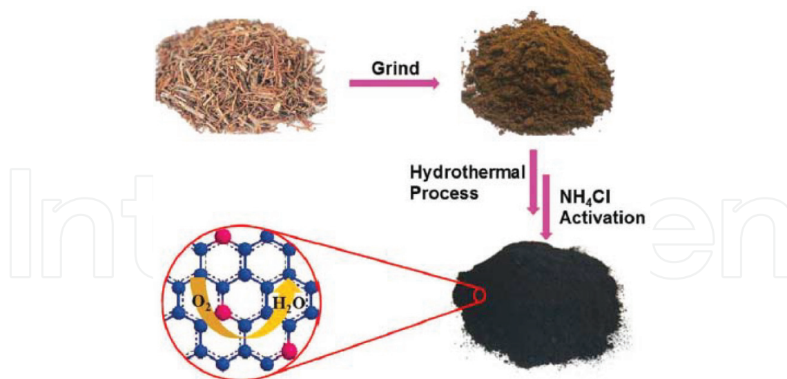
Figure 5. Schematic procedure for the synthesis of heteroatom doped porous carbon materials derived from Gentiana scabra Bunge [70].
