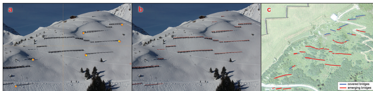
Figure 8. Snow bridges (Adelboden, 2018). (a) Original oblique image of the snow bridge constructions with control points. (b) Digitalization of the snow bridges. (c) Projection of the digitalized bridges on the current orthophoto highlighting in blue the parts covered by snow.
