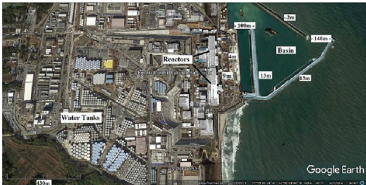
Figure 1. Top view of Fukushima power plant Dezember 2015 with lateral and height dimensions.
