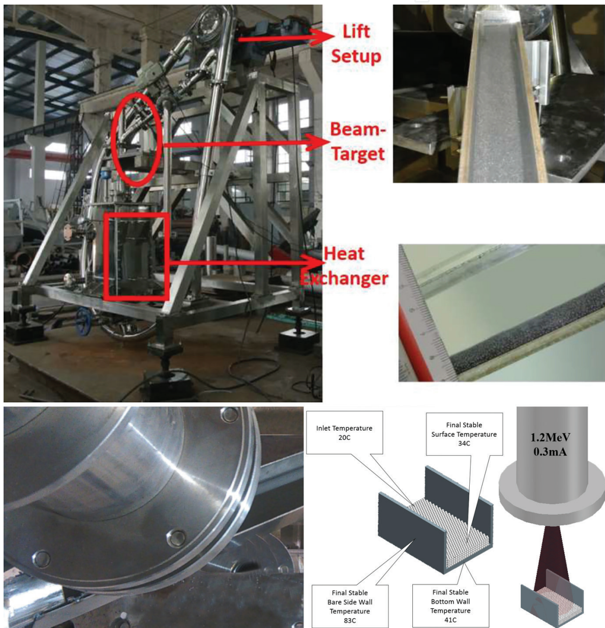
Figure 6. Electron beam coupling of chute flow target.
