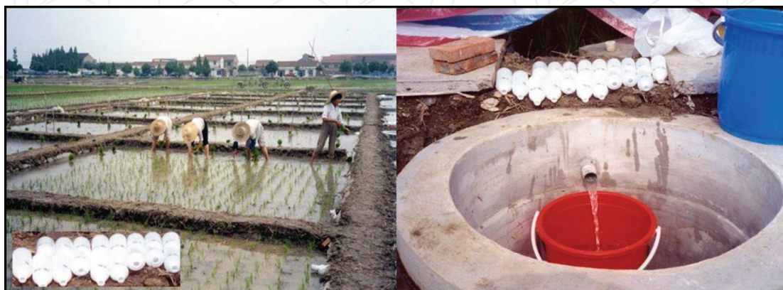
Figure 6. Monitoring of water quality in paddy systems: Research plots and field ponding water on the left and runoff collection facility on the right.
