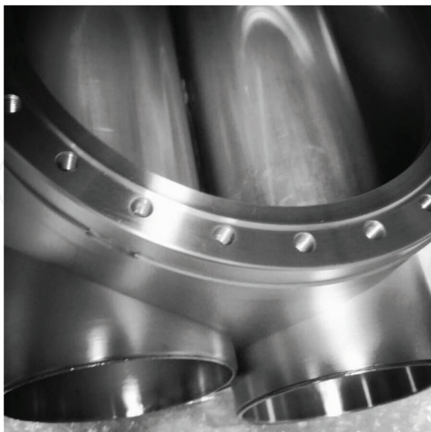
Figure 4. Detail of the lower chamber of the UHV vacuum system, showing the two thin steel tubes that allow management of field masses without feedthroughs by keeping them outside the vacuum vessel.
