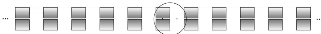
Figure 5. Scheme of the periodic field mass principle. Rest positions of the two bobs are shown (black dots). The circle in the middle represents the outline of the lower vacuum chamber through whose tunnels, shown in Figure 4 , the field mass systems go.
