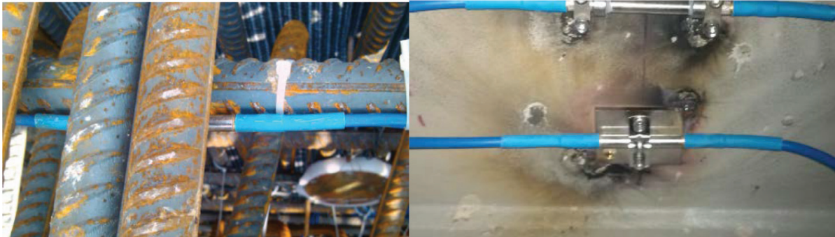
Figure 14. Installation diagram of FBG temperature sensor.
