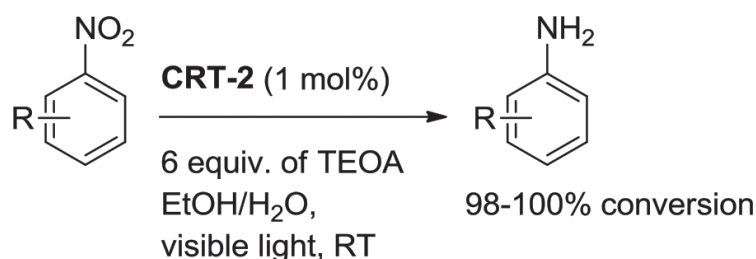
Scheme 3. (CRT-2) catalyzed photoredox conversion of nitrobenzene to aniline.
