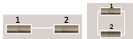
Figure 7. Illustration of system, combined from series (left) or parallel (right) elements.
