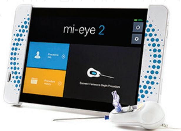
Figure 1. Device. The mi-eye 2 device from trice medical, which includes the tablet and disposable probe. The needle sheath is retracted by pushing back on button found on superior portion of device.
