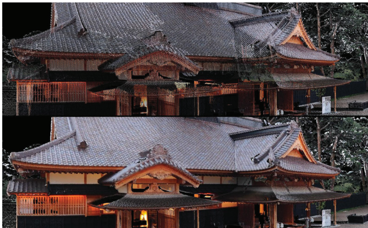
Figure 6. LiDAR VR processing result: input point cloud (upper image) and output point cloud (bottom image).
