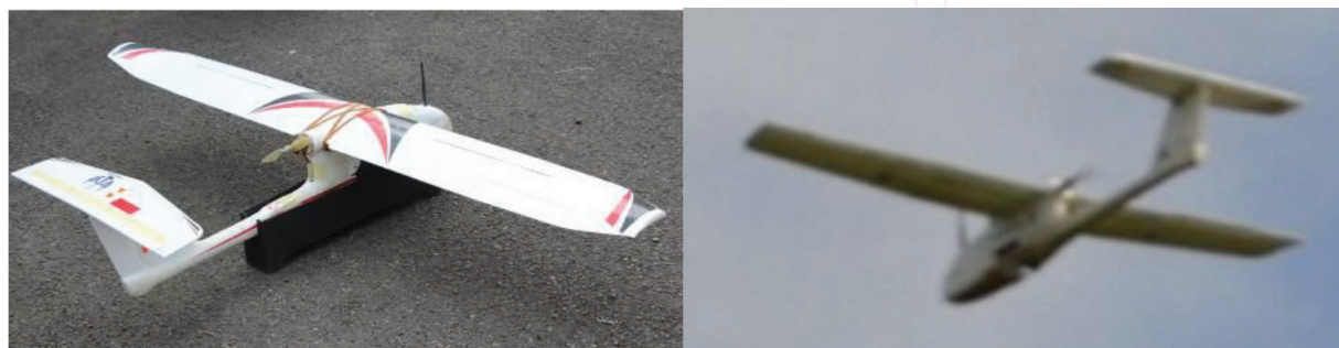
Figure 4. Left: LSU-01 final configuration; right: LSU-01 during operation with the camera bay shown under the fuselage.
