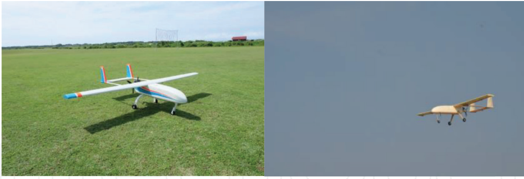
Figure 6. Left: LSU-03 final configuration shortly before takeoff; right: LSU-03 test flight.
