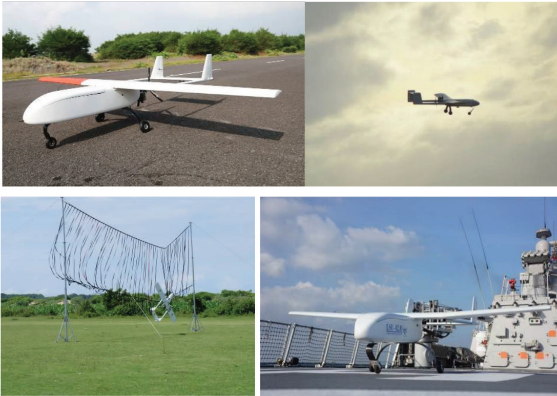
Figure 5. Top-left: LSU-02 final configuration shortly before takeoff; top-right: LSU-02 during aerial photography mission; bottom-left: landing operation with net; bottom-right: takeoff preparation from Indonesian Hasanudin class corvette warship.
